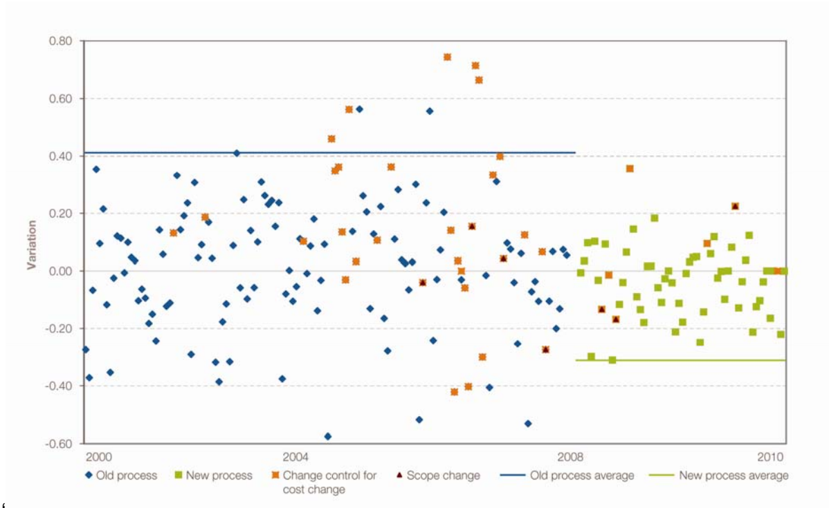
Figure 4: Comparison of actual cost versus estimated cost using old (pre-2008) and revised (2008 – 2010) estimation process
