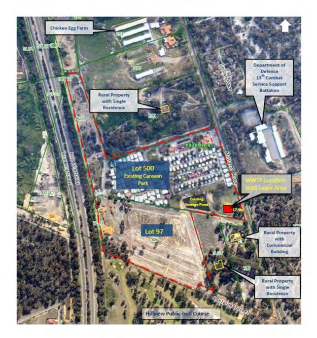
Both Lots 97 and 500 sites currently have no Water Corporation sewerage services available. The existing BTP has a sewerage pipe network that is serviced by an existing open pond aerobic waste treatment system. Connection to the municipal sewer network is not feasible and will financially jeopardise the development of FLV. BW further proposes to redevelop the existing BTP in part at some time in the future.
