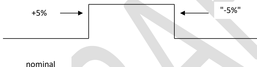
Fig A11-1 - Application of step signal
