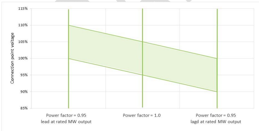
Figure 3-3 Relaxation of reactive power requirement with connection point voltage
