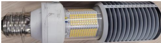
Figure 1: An example of an LED lamp with extensive parts that will not allow light to pass through.
